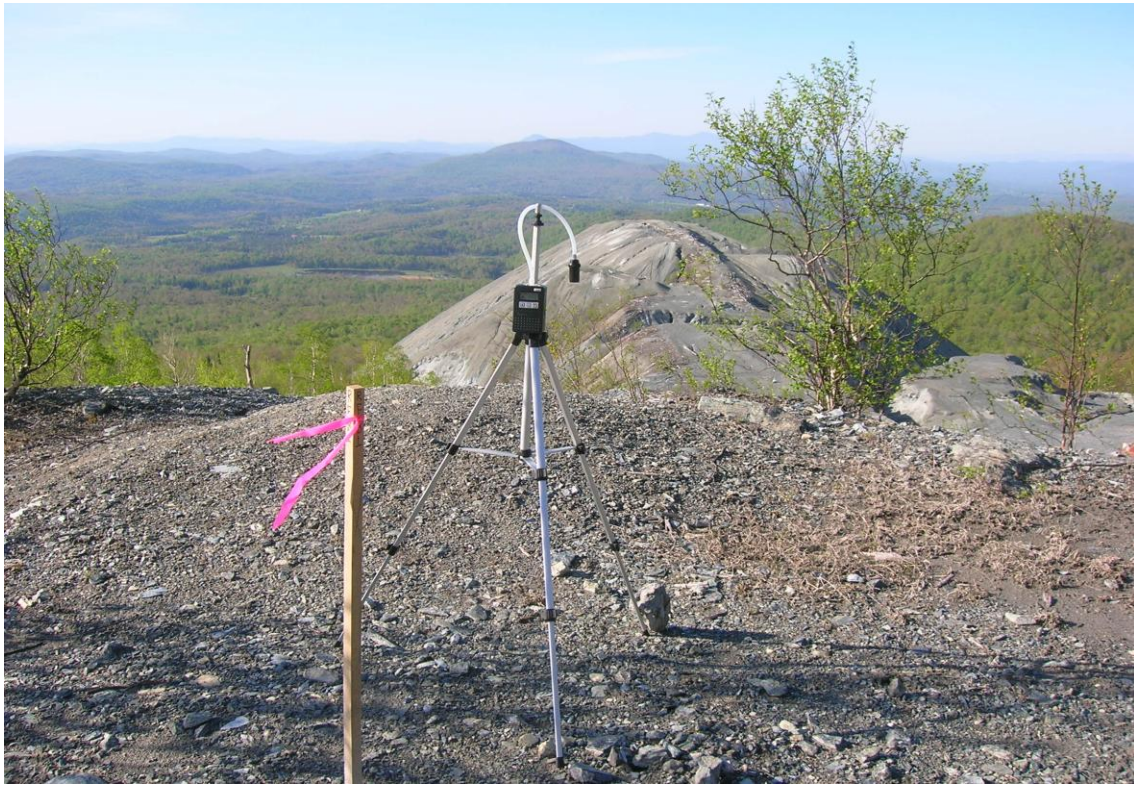
Air Monitoring Station on the Eden Quarry testing for airborne asbestos fibers
